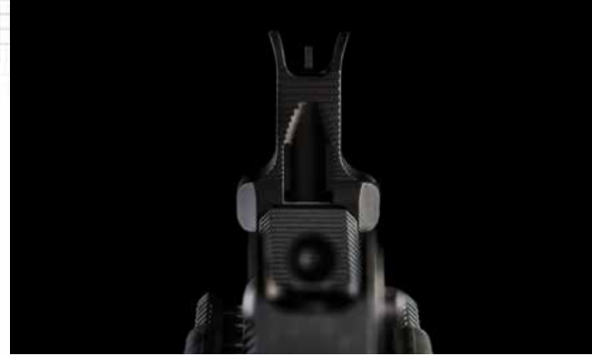
The DDM4 Rail™ 15.0 provides the V9 with a long sight radius for precision shooting with iron sights. The long expanse of Picatinny rail allows the user to customize exactly where accessories are mounted.
