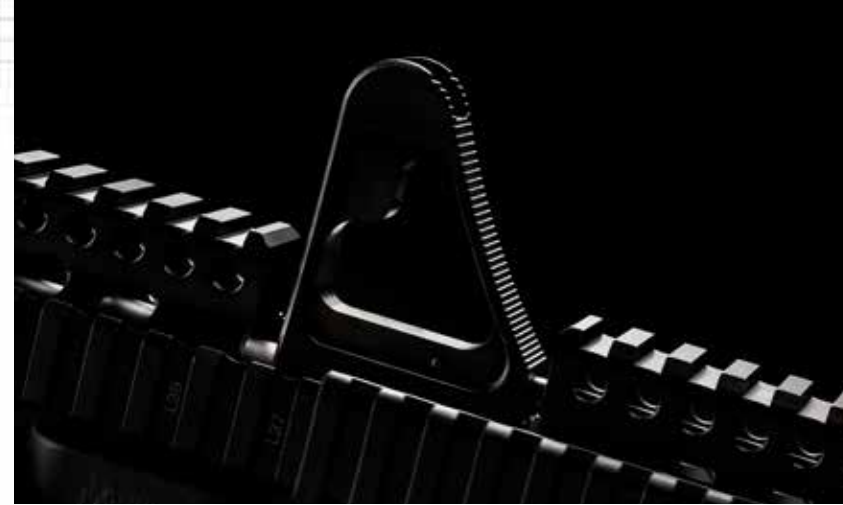
One of the V1's most visible attributes is its proprietary front sight base, CNC-machined from 4140 steel, finished with a salt bath nitride surface treatment, and featuring a serrated curved design to minimize glare.
